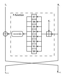
Parameters: K - session key (256 bit) S-boxes - long-term key (512 bits) Input/Output = 64/64 bits Cipher based on Feistel Network with r = 32 rounds.
